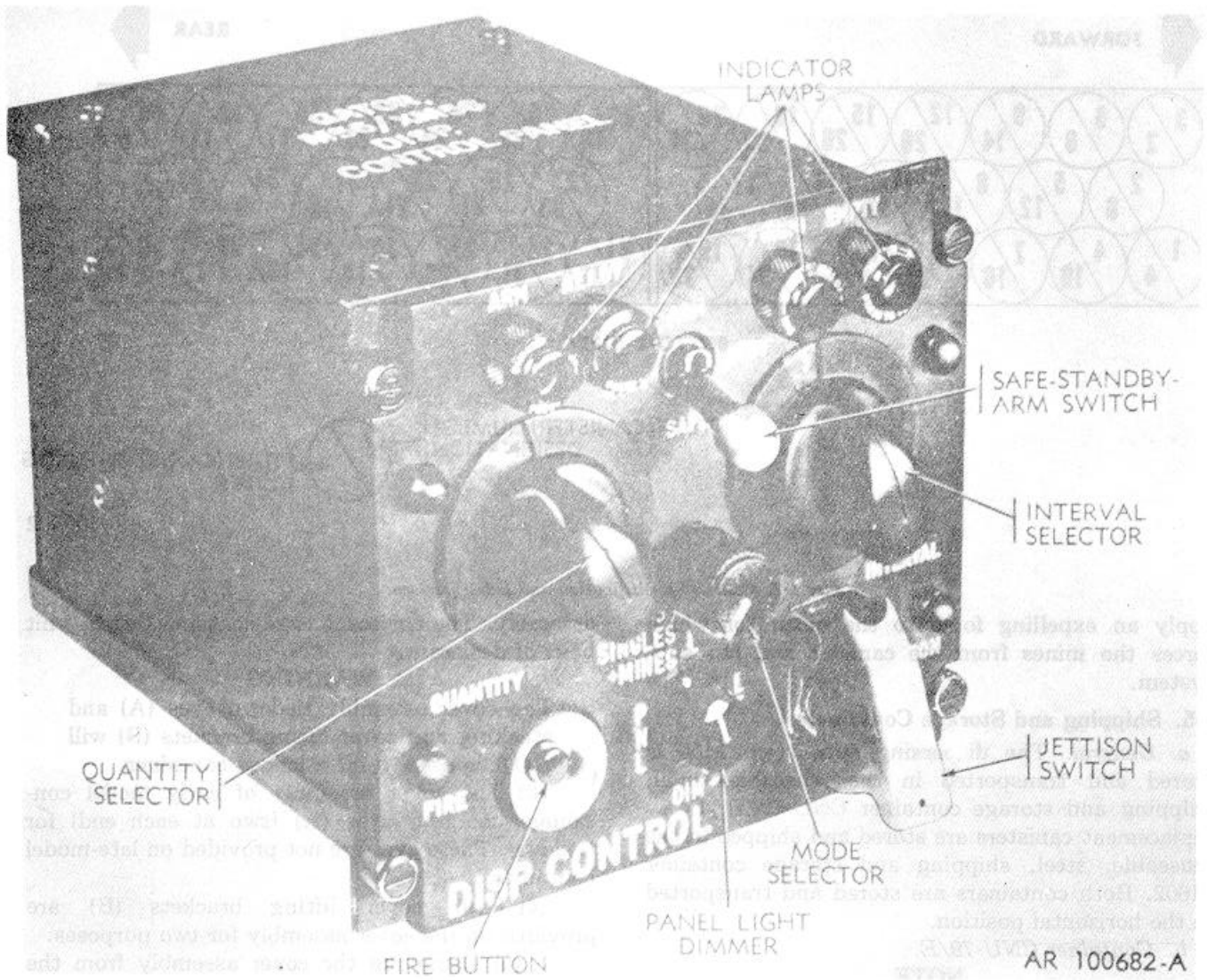
Figure 1-6. Mine dispersing subsystem M56 dispenser (DISP) control panel.
